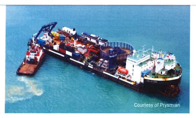
No oil-based insulation is used in the design of these cables meaning no leakage in the event of damage to the cables. The submarine sections of the cables have additional armouring to provide mechanical protection as they are delivered off the back of a cable-laying vessel directly onto the seabed.
